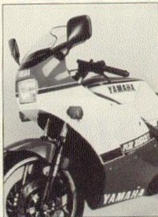
Front end gets clip-on bars, new fork and opposed-piston caliper brakes.
