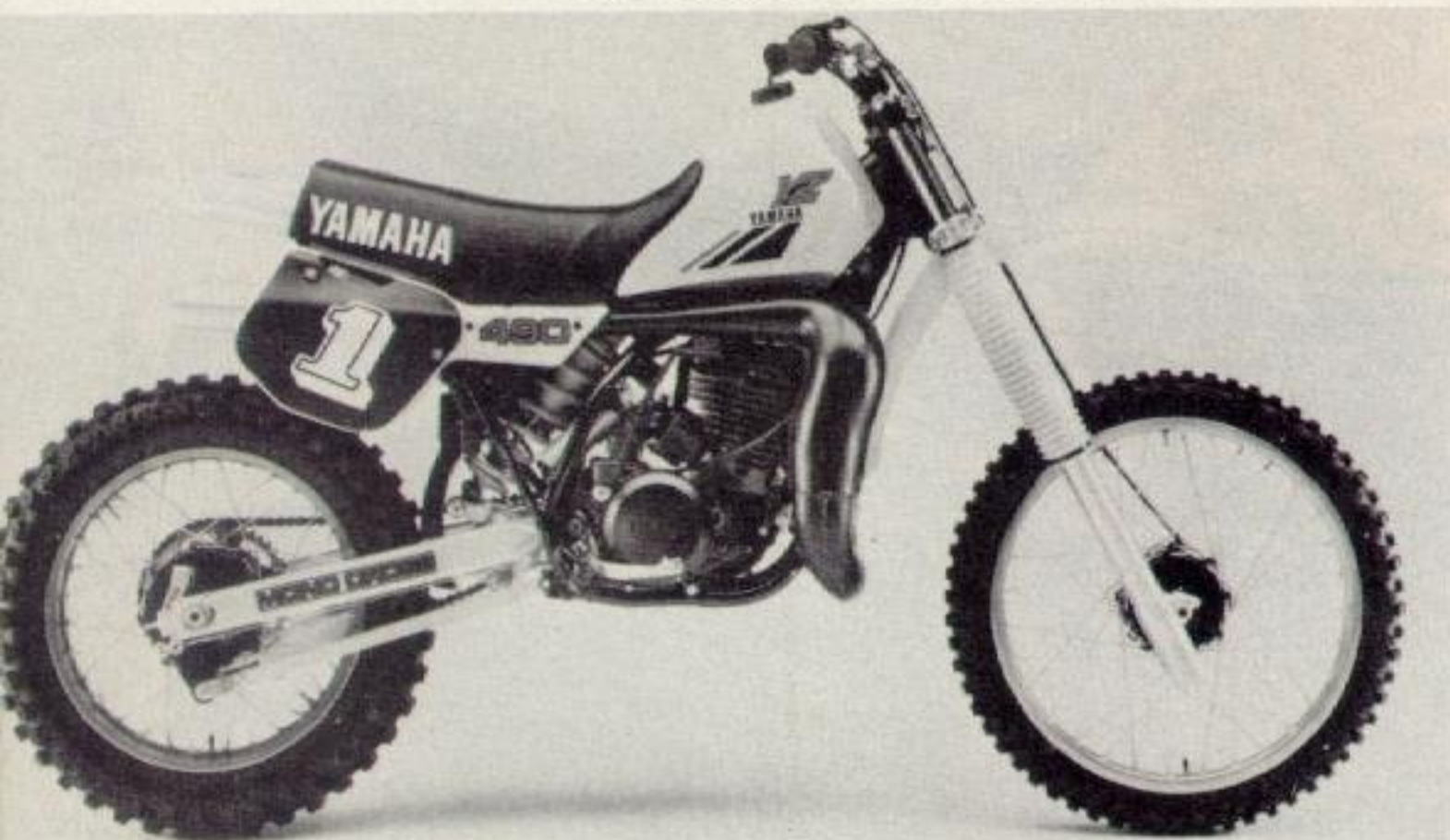
YZ490 has more power with a new pipe, 40mm carb. and porting changes. Forks now have compression damping and rear suspension is revised. All '84 motocrossers have new Z-spokes.
