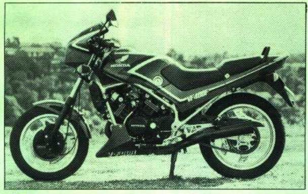
Water-cooled 90 degree V four four-stroke, crankshaft set transversely Double overhead camshaft driven by HyVo chain, four valves per cylinder. Barrels cast integrally with top of crankcase. One-piece crankshaft, plain main and hig end bearings. Wet sumn lubrication.
